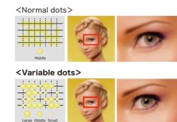
Dots are combined with the minimum size of 4pl to enable smooth color printing with less granular feeling.
