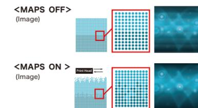
Based on printing conditions such as media/ink type and resolution, the most suitable gradation pattern is automatically selected and printed.
