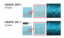
Based on printing conditions such as media/ink type and resolution, the most suitable gradation pattern is automatically selected and printed.
